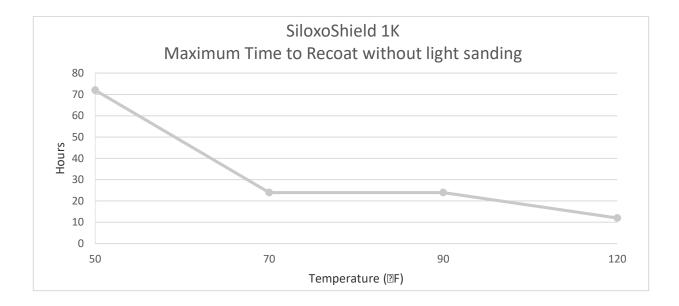
Sanding required above the line of the recoat graph. No Sanding required below the line of the recoat graph.
